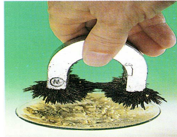
FIGURE 1.9 Formation of a mixture is a physical change. Here we see that forming the mixture has not changed the iron and sulfur into a compound of these two elements. The mixture can be separated by pulling the iron out with a magnet.
