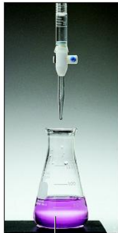
(c) When the amount of NaOH added from the buret exactly equals the amount of H^+ supplied by the acid being analyzed, the dye (indicator) changes color.
